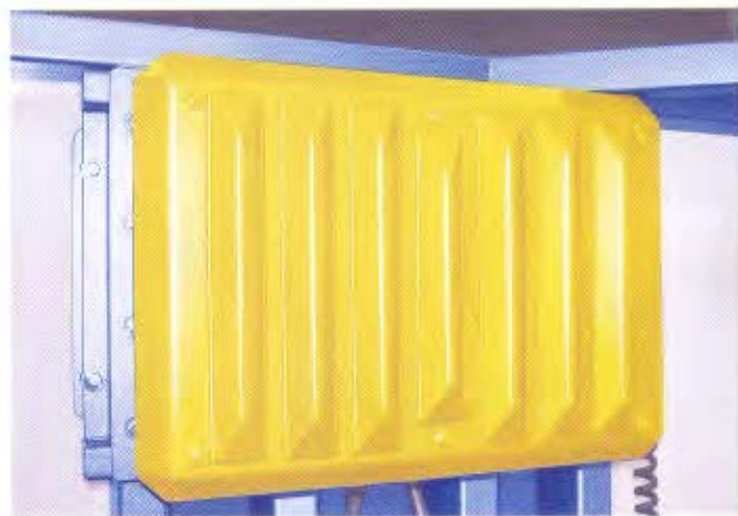
Hydraulic conditioning plates on opposing sides of the bag loosen the material.
