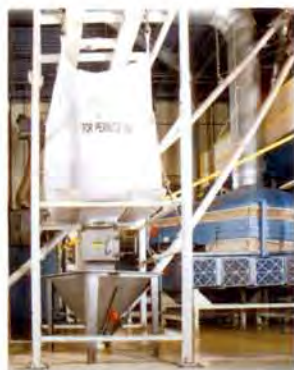
Two bulk bag unloaders, each with a 25 ft (7.6 m) long flexible screw conveyor, maintain a continuous flow of shelled peanuts to the gas-fired roaster in background. The fully enclosed system enhances plant sanitation and reduces manual handling.
