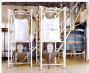
Two bulk bag unloaders, each with a 25 ft (7.6 m) long flexible screw conveyor, maintain a continuous flow of shelled peanuts to the gas-fired roaster in background. The fully enclosed system enhances plant sanitation and reduces manual handling.
