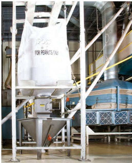
► One of the two bulk bag unloaders installed at Nutco is shown here. Each has a 25-ft. (7.6 m)-long flexible screw conveyor and maintains a continuous flow of shelled peanuts to the gas-fired roaster in the background. Source: Flexicon.
