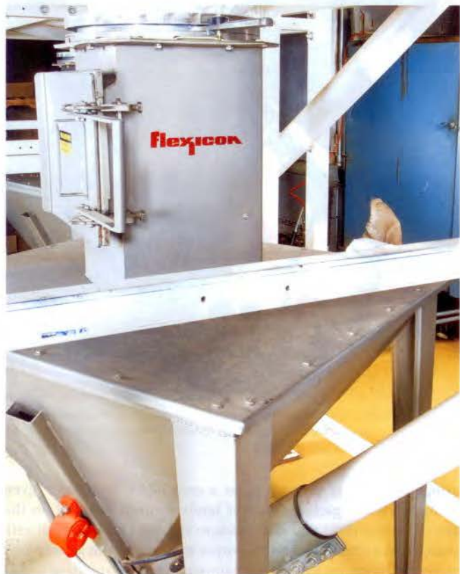
Peanuts are discharged from the bulk bag into the receiving hopper through a manually operated 305 mm dia iris valve attached to the bag spout.
