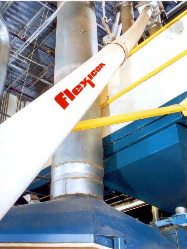
Each 7.6 m long flexible screw conveyor consists of a rotating, stainless steel spiral screw, housed in a 115 mm o.d. polymer tube.
