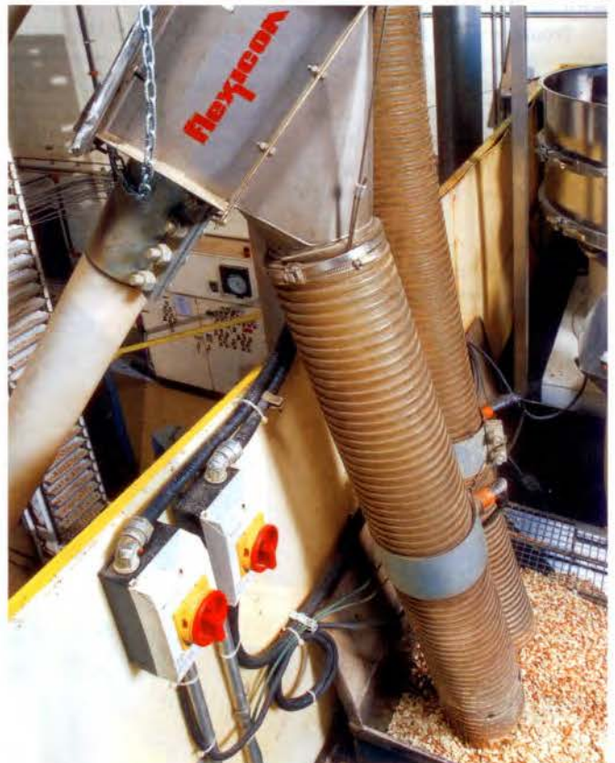
Each flexible screw conveyor empties peanuts (through a discharge adapter and flexible downspout) into a surge hopper from which they are conveyed to the roaster.
