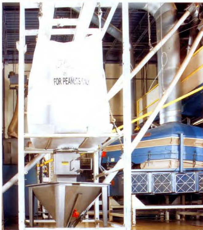
Two bulk bag unloaders, each with a 7.6 m long flexible screw conveyor, maintain a continuous flow of shelled peanuts to the gas-fired roaster in background. The fully enclosed system enhances plant sanitation and reduces manual handling.
