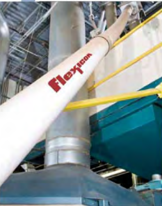
Each 7.6m long flexible screw conveyor consists of a rotating, stainless steel spiral screw, housed in a 115mm o.d. polymer tube.
