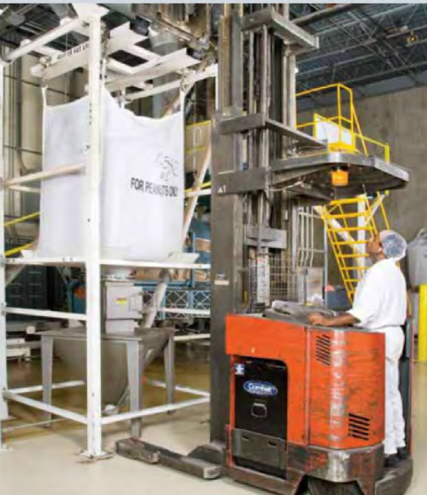
Operator forklift-loads bag-lifting frame onto the bulk bag unloader.
