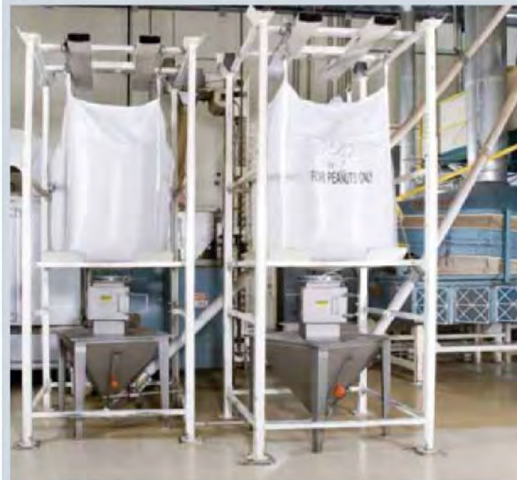
Two bulk bag unloaders, each with a 7.6m long flexible screw conveyor, maintain a continuous flow of shelled peanuts to the gas-fired roaster in background. The fully enclosed system enhances plant sanitation and reduces manual handling.
