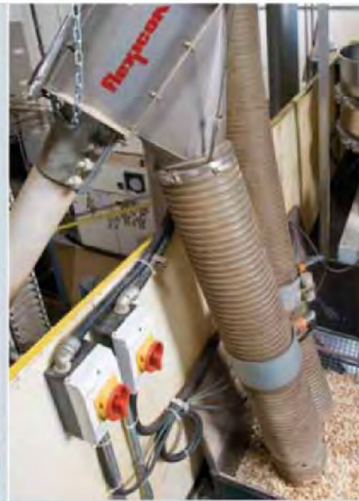
Each flexible screw conveyor empties peanuts (through a discharge adapter and flexible downspout) into a surge hopper from which they are conveyed to the roaster.
