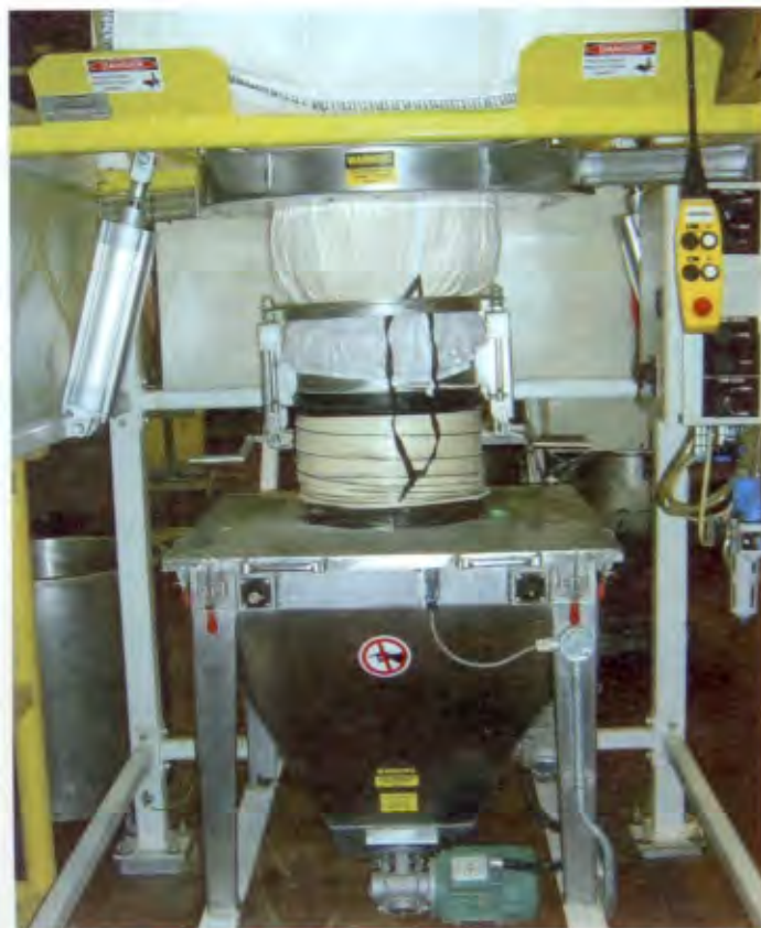
Spout-Lock and Tele-Tube, bulk bag spout interface enabling a quick, dust-tight connection between the bag spout and receiving hopper
