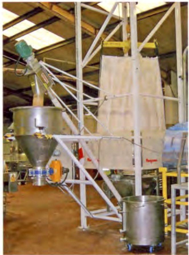
ABOVE: Flexicon's bulk bag discharge system made ready to transfer dry recipe into mixer vessels for the depositor line
