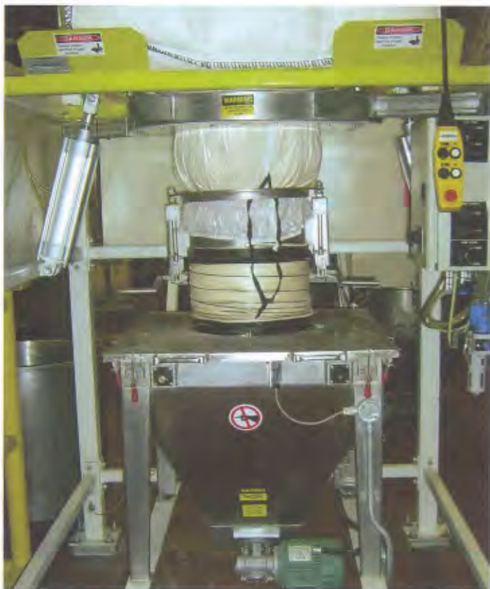
Spout - Lock and bulk bag spout interface enabling a quick, dust-tight connection between the bag spout and receiving hopper
