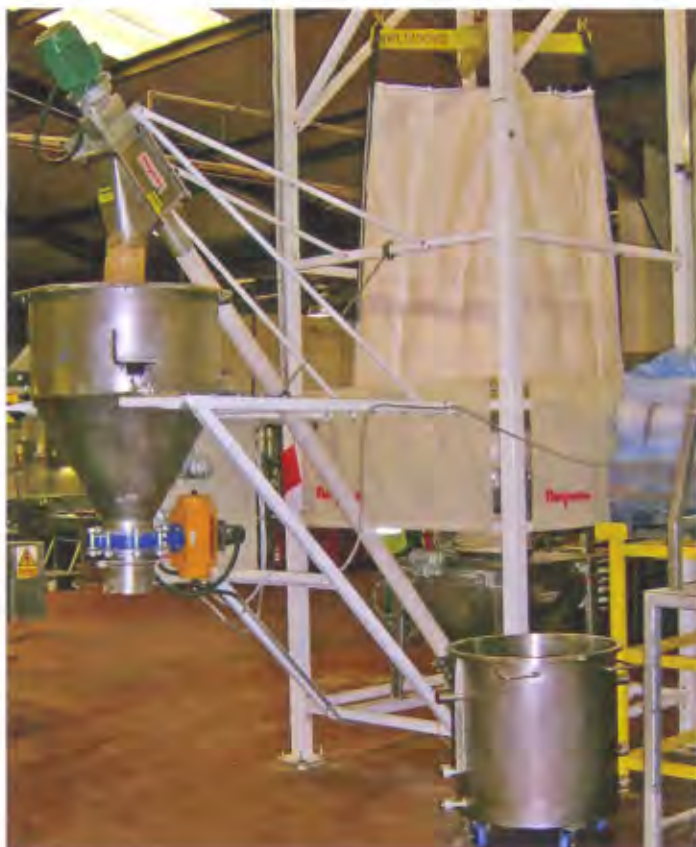
Flexicon's Bulk Bag Discharge System made ready to transfer dry recipe into mixer vessels for the depositor line
