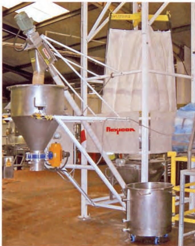
The bulk bag weigh-batching system conveys dry ingredients from the bulk bag to a gain-in-weight hopper that discharges it into mobile wet mixing vessels.
