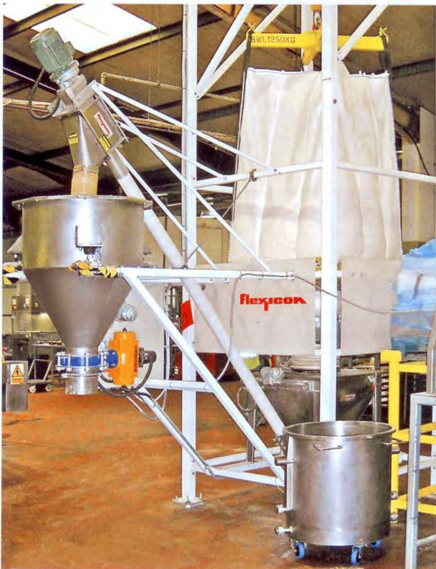
Bulk bag weigh batching system conveys dry ingredients from bulk bag to a gain-in-weight hopper that discharges into mobile wet mixing vessels.
