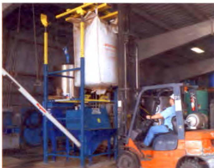
Forklift operator positions bag lifting frame on top of the bulk bag unloader
