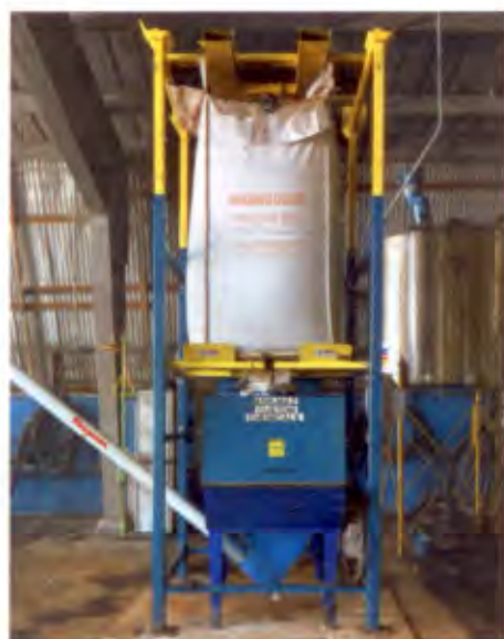
Cradle at top of the bulk bag unloader supports the removable bulk bag lifting frame
