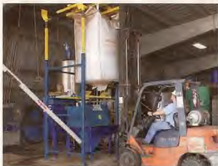
The removable bulk bag lifting frame is lifted and positioned using a forklift truck.
