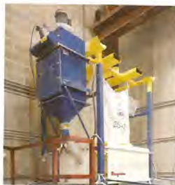
A Bag-Vac® dust collector, mounted on the bulk bag unloader frame, vacuums displaced air and dust, and collapses empty bags dust-free prior to tie-off and removal. The bulk bag is supported in a lifting frame.
