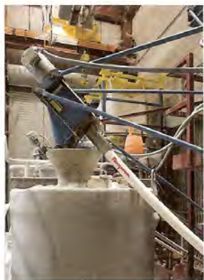
DE transferred by the flexible screw conveyor is discharged into a tank, where it is put in suspension with water
