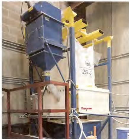
A Bag-Vac dust collector vacuums displaced air and dust, and collapses empty bags prior to tie-off and removal
