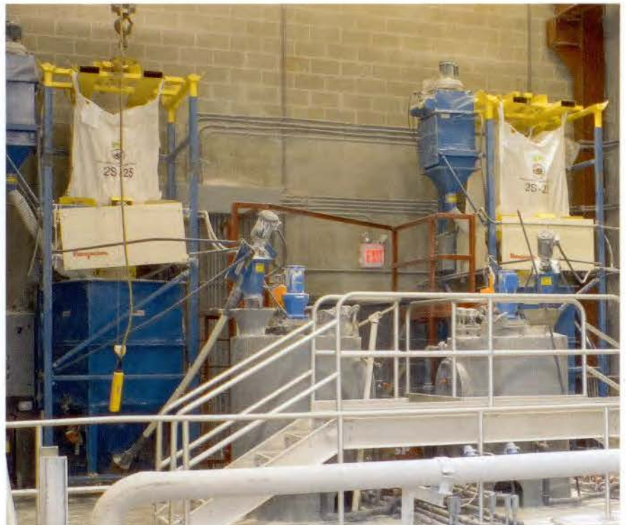
The two independently operated batch weighing and dosing systems can feed diatomaceous earth from bulk bags into a filter tank at up to 10 ft 3 /h.
