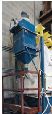
**Right: At the flexible screw conveyor's discharge end, DE flows through a transition adapter into the 1136 L tank where the DE is put in suspension with water**
