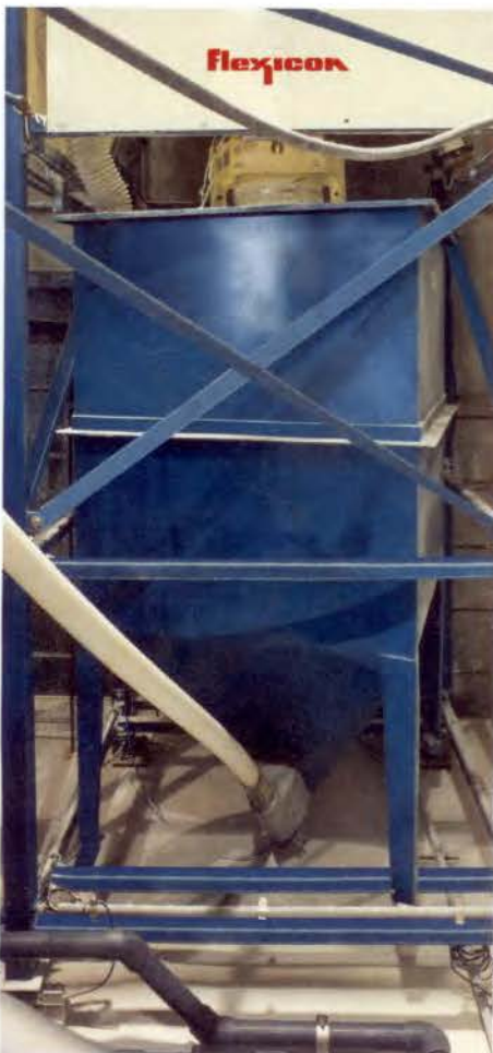
One of two 1.8m 3 capacity hoppers holds the contents of a 408 kg bulk bag allowing diatomaceous earth to transfer, unattended, through the flexible screw conveyor to the tank. Load cells under the unloader frame transmit weight loss information to a PLC to achieve accurate batch weight transfer.
