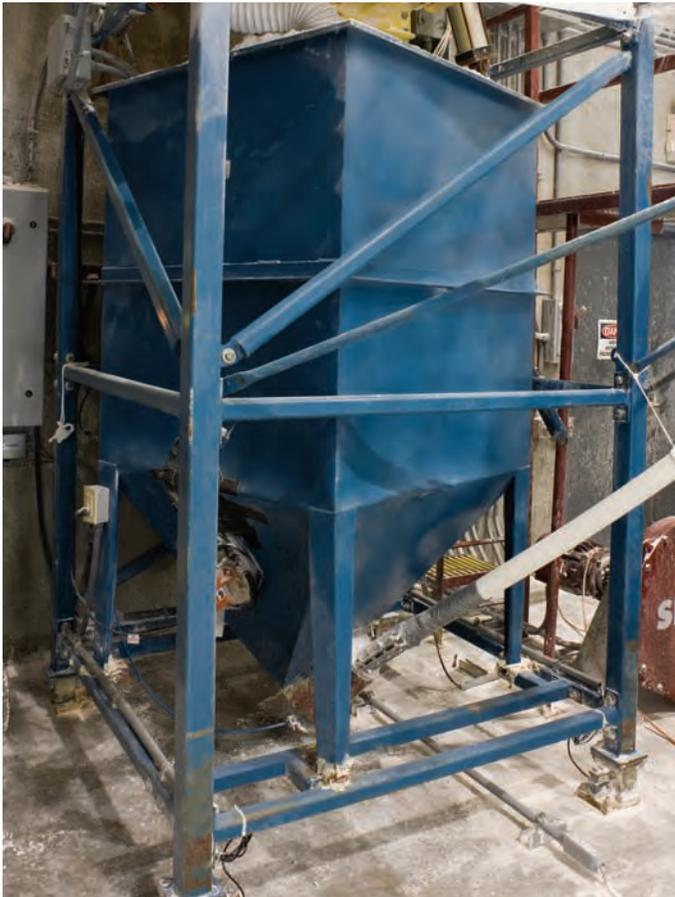
*Figure 4: The 63 cu ft (1.8 cu.m) Capacity Hopper Holds the Contents of a 900 lb (408 kg) Bulk Bag Allowing Diatomaceous Earth to Transfer, Unattended, through the Flexible Screw Conveyor to the Tank. Load Cells Under the Unloader Frame Transmit Weight Loss Information to a PLC to Achieve Accurate Batch Weight Transfer.*
