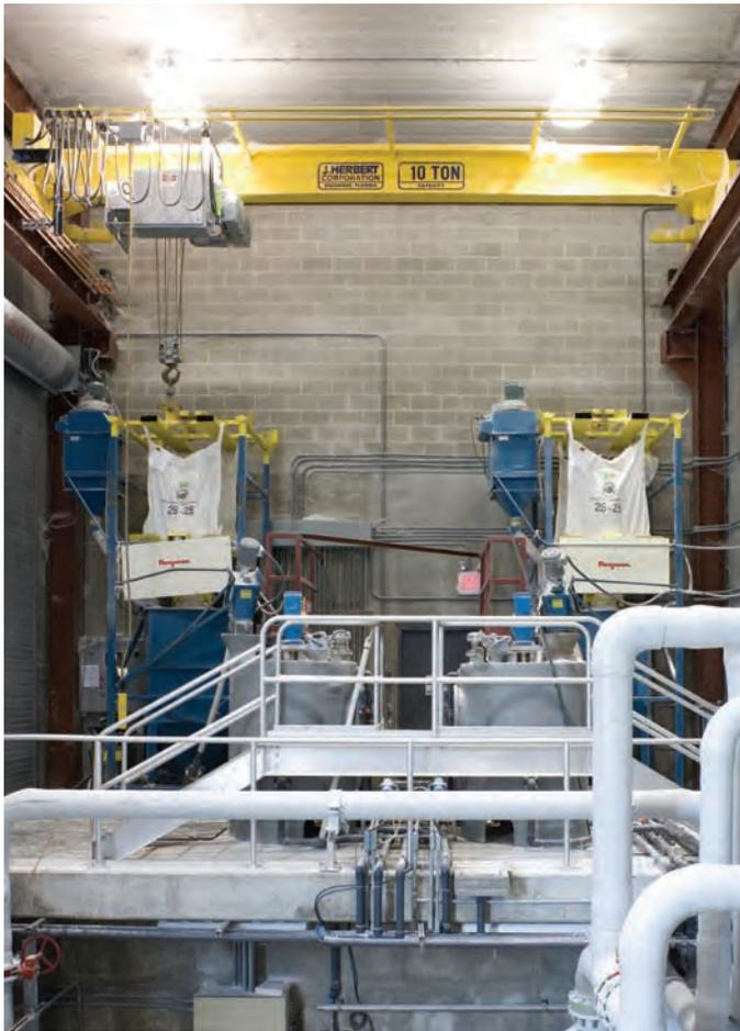
Figure 2: Two Bulk Bag Unloaders Unload and Transfer 4000-6000 lb (1814-2722kg) Per Day of Diatomaceous Earth (DE) for Tampa Bay desalination plant's DE Filtration System. The Crane Deposits a Lifting Frame Holding the Bulk Bag onto the Unloader Frame.
