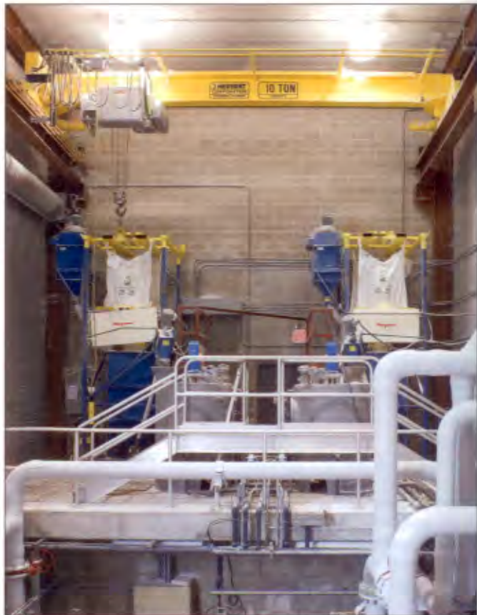
Above and Below: Two bulk bag unloaders unload and transfer 1814-2722 kilograms per day of diatomaceous earth for Tampa Bay desalination plant's diatomaceous earth filtration system. The crane deposits a lifting frame holding the bulk bag onto the unloader frame.
