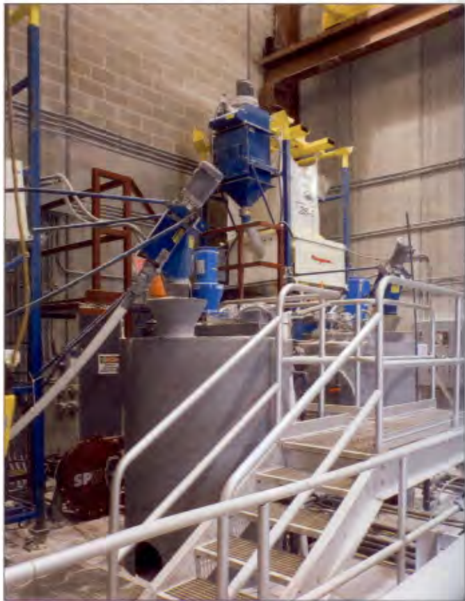
Above and Below: Two bulk bag unloaders unload and transfer 1814-2722 kilograms per day of diatomaceous earth for Tampa Bay desalination plant's diatomaceous earth filtration system. The crane deposits a lifting frame holding the bulk bag onto the unloader frame.
