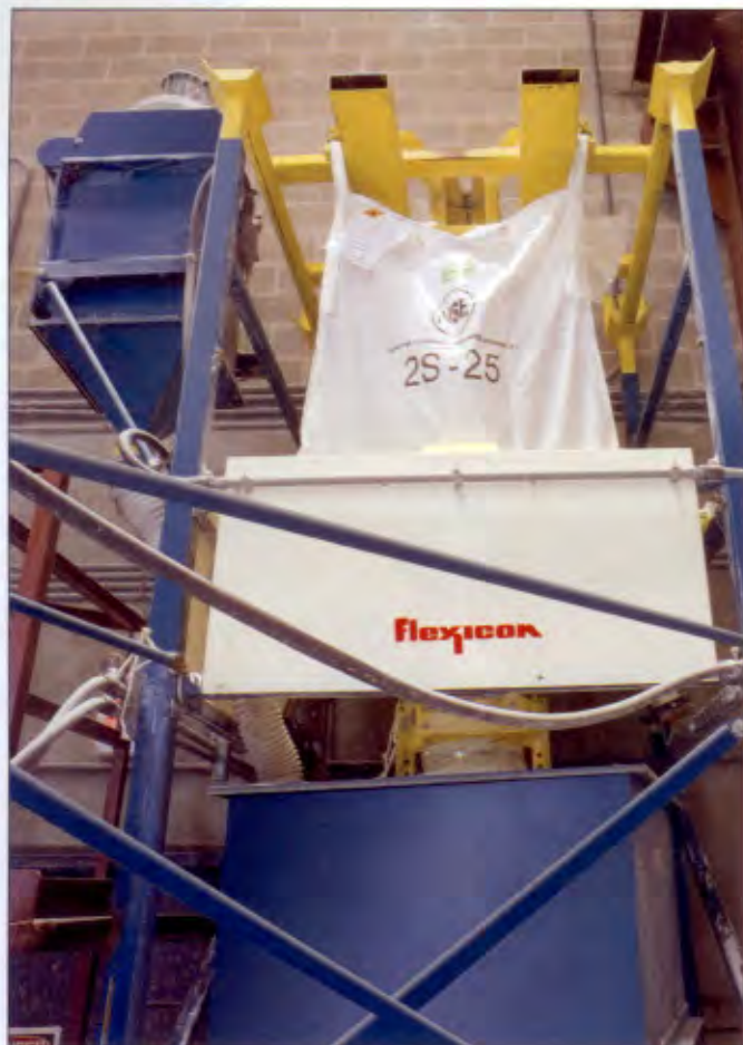
Above and Below: A Bag-Vac dust collector, mounted on the bulk bag unloader frame, vacuums displaced air and dust, and collapses empty bags dust-free prior to tie-off and removal. The bulk bag is supported in a lifting frame.
