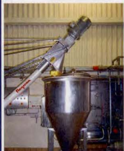
The flexible screw conveyor moves the free-flowing raw material 14.8 ft (4.5m) at a 45-degree incline into a hopper.
