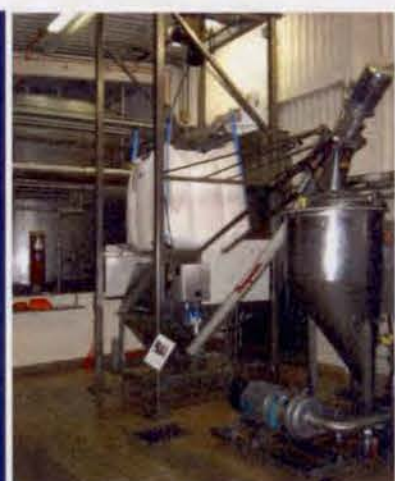
The new bulk bag discharger system at Danisco covers a small footprint while reducing costs and waste.
