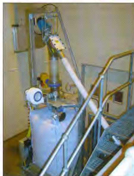
The FIBC on the Bulk Bag Filler Frame in readiness for transfer to the discharge line for bagging or shipment as an FIBC load
