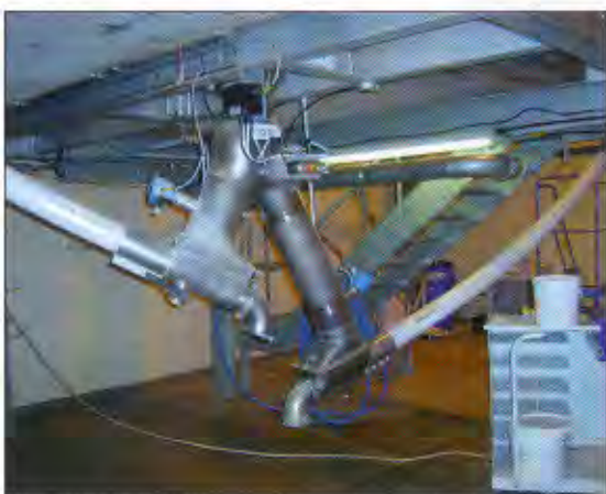
Two flexible screw conveyors offer the choice of either directing flow primarily into the bagging line or, in the event of a line problem, into a 1-tonne flexible intermediate bulk container (FIBC)
