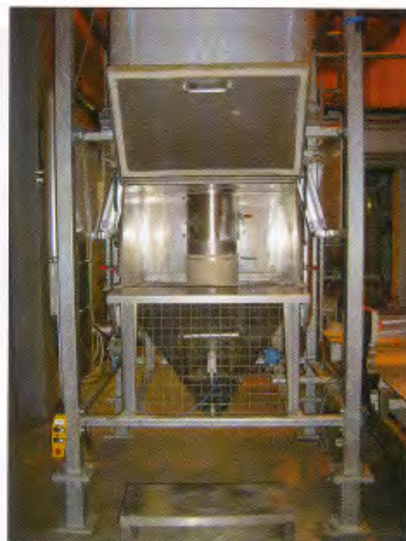
The discharge receiving hopper with open hood showing access to the bag spout and iris valve
