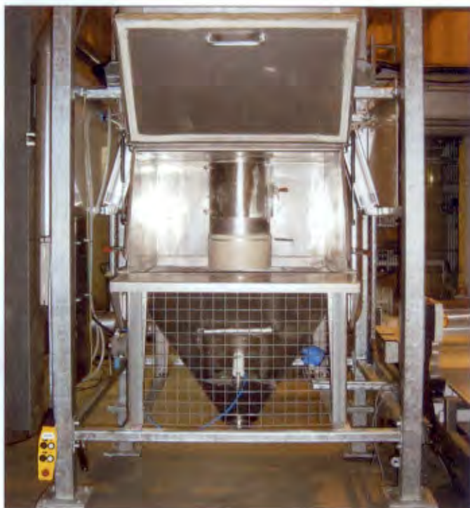
Opening a door on the hopper intake chute of the bulk bag discharger frame exposes the bag spout
