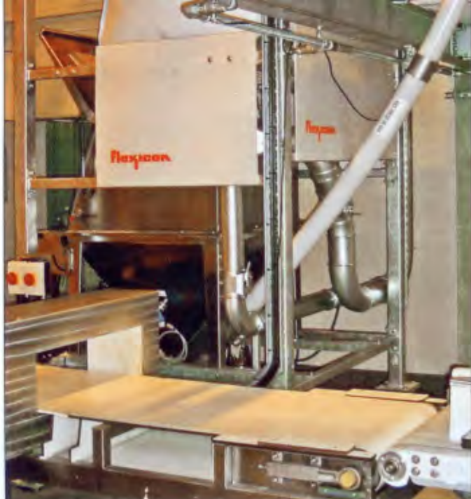
This bulk bag discharger with integral flexible screw conveyor moves malt from bulk bags to the bagging line.
