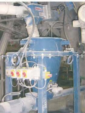
The upper flexible screw conveyor transfers aluminum powder from the bag dump station to the top of a weigh hopper, while the conveyor below feeds weighed batches to the blender.
