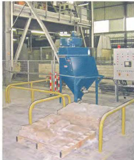
The upper flexible screw conveyor transfers aluminum powder from the bag dump station to the top of a weigh hopper, while the conveyor below feeds weighed batches to the blender.
