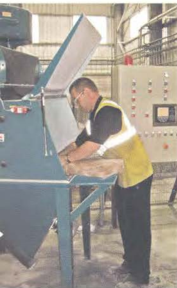
Dust generated by splitting and dumping of bags is contained by a dust collector at the bag dump station.
