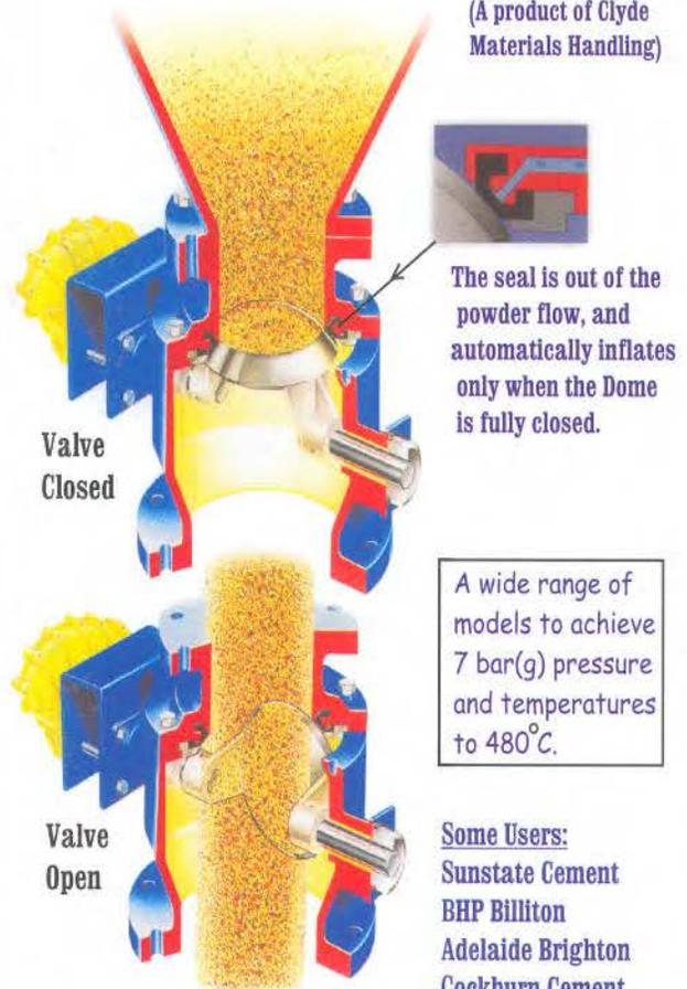
The seal is out of the powder flow, and automatically inflates only when the Dome is fully closed.
