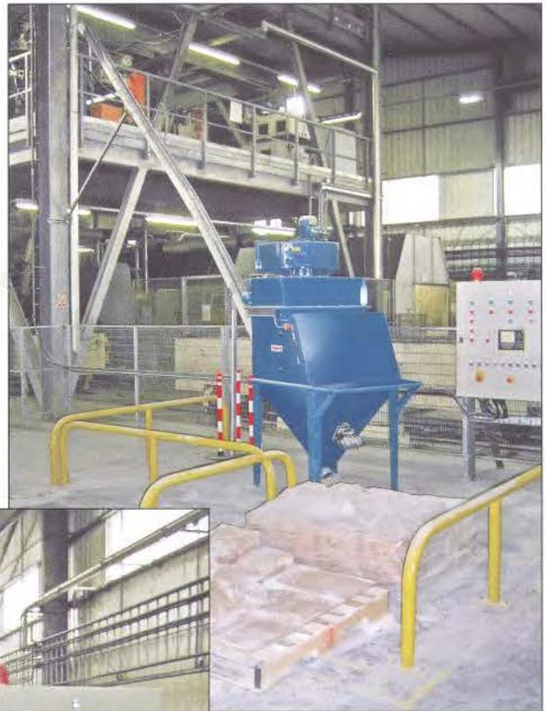
*A nine-metre-long flexible screw conveyor transfers aluminium powder from a bag dump station to a gain-in-weight hopper on the mezzanine.*
