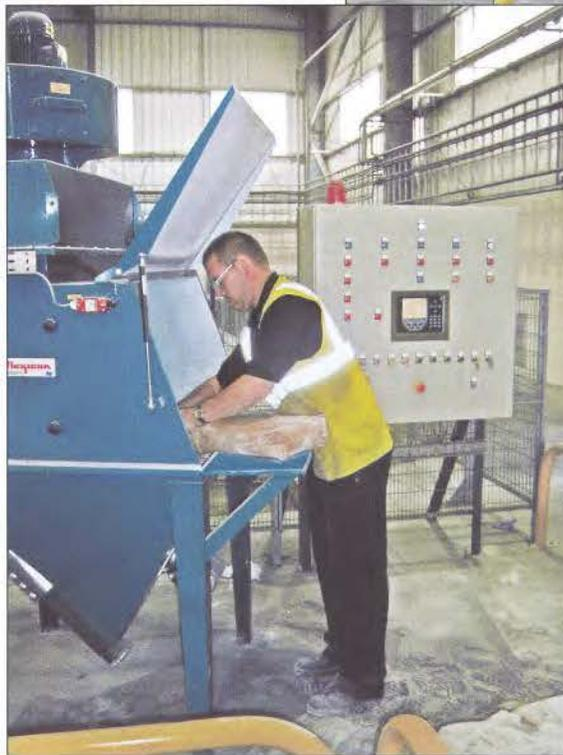
***The weighing, transferring and unping of material by one operator required two hours and generated dust, calling for an overhaul of the process.***
