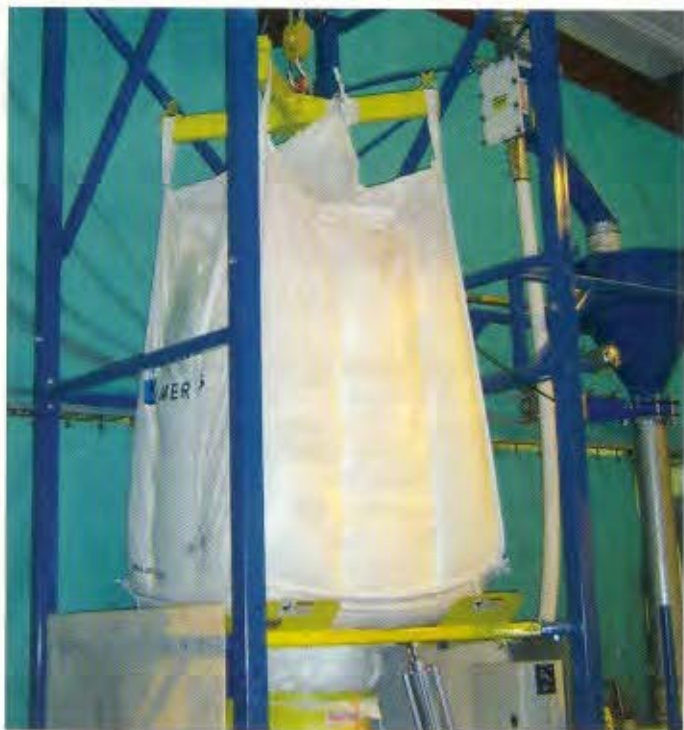
ABOVE: The bulk bag mounted in the frame ready for discharge into the receiving hopper via the Tele-Tube assembly
