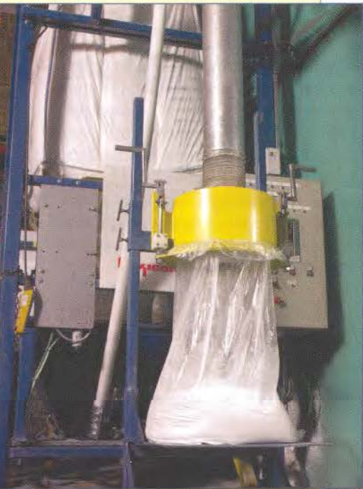
Cumberland's colored pencil production meant dealing with China clay, which caused an airborne dust problem within the plant.
