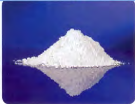
China clay makes a pretty reflection in repose, but can cause airborne dust when it is transferred in the open
