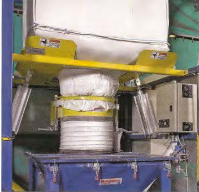
The Spout-Lock clamp ring and Tele-Tube telescoping tube allow a quick, dust-tight connection between the bag spout and the hopper and elongate the bag as it empties, thereby promoting flow.
