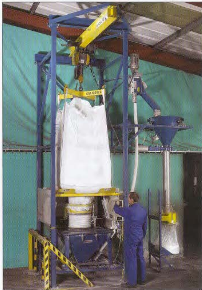
Figure 1: A bulk bag is mounted in the frame, ready to discharge clay into the receiving hopper via the Tele-Tube assembly.
