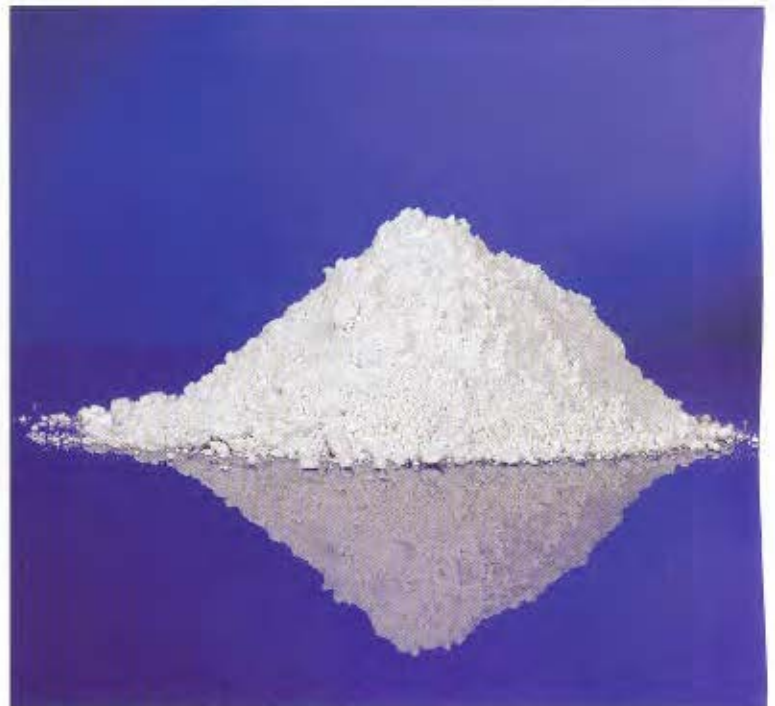
Figure 5: China clay makes a pretty reflection in repose, but can cause airborne dust when it is transferred in the open.
