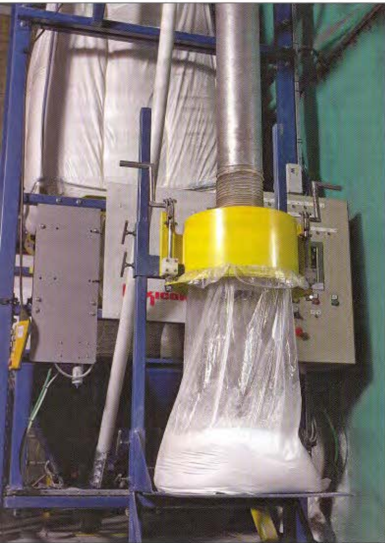
Figure 4: When the weigh hopper reaches its target weight, the batch of clay is discharged into a bag and taken to the blender.
