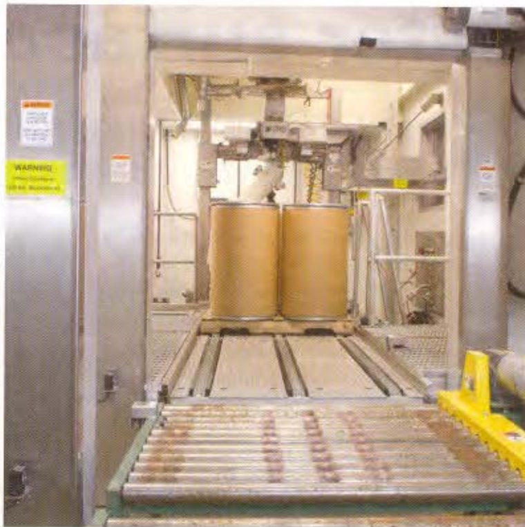
Pallet of four drums is conveyed into purpose-built loading room where they are filled by rotating drum/bulk bag filler
