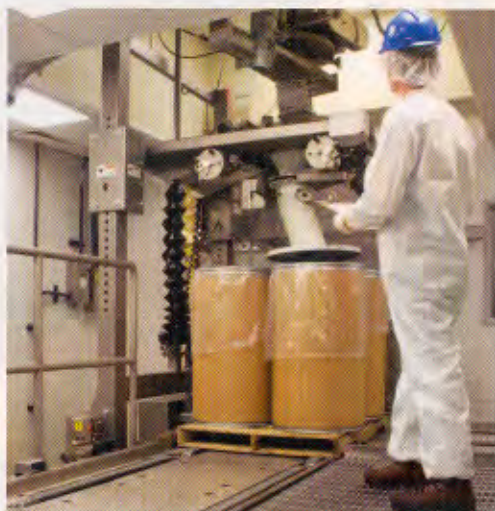
Filled drums are conveyed from loading room to shipping area.
