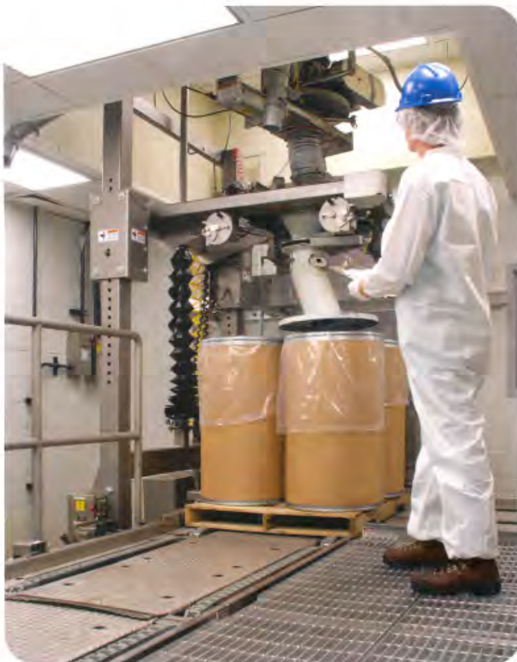
Automated drum filler utilizes an indexing diverter head to fill four 55 gal (208 liter) drums sequentially with surfactant powder gravity feeding from rotary valve at top. System can also be configured for loading 2000 lb (907 kg) bulk bags.
