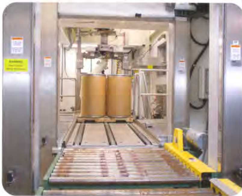
Pallet of four drums is conveyed into purpose-built loading room where they are filled by rotating drum/bulk bag filler.
