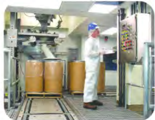
PLC communicates with weigh-filler scale to regulate product flow into each drum and shut down on reaching a pre-set weight. Four drums await filling as four are about to exit the room. System improves product output, worker safety, and quality control.
