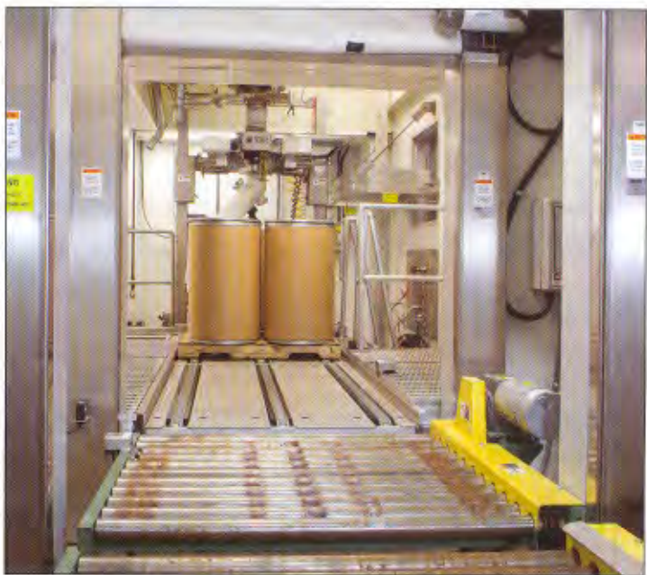
Pallet of four drums is conveyed into purpose-built loading room where they are filled by rotating drum/bulk bag filler.
