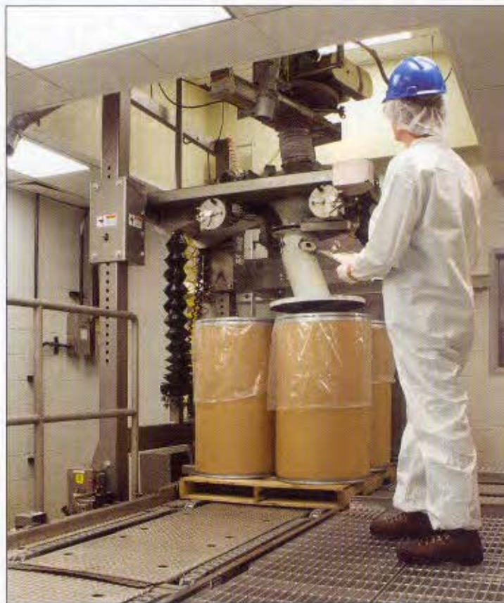
Automated drum filler utilises an indexing diverter head to fill four 208 litre drums sequentially with surfactant powder feeding from rotary valve at top. System can also be configured for loading 907-kg bulk bags
