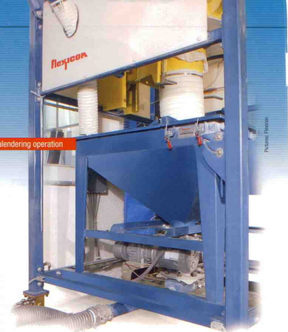
Below the hopper on the bulk bag discharger frame, a drop-through rotary valve meters PVC resin into two pneumatic conveying lines.
