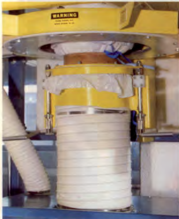
At the bag-spout interface , a clamp ring creates a dust-tight seal while a telescoping tube maintains constant downward pressure as the bag empties to promote discharge.
