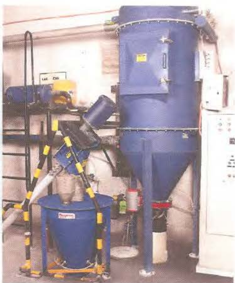
Fig. 3: A Flexicon flexible-screw conveyor empties calcium carbonate into the smaller weigh hopper. Both ingredients are then gravity fed to the mixer on the floor below.
