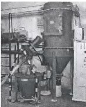
PVC from the bulk bag unloader is pneumatically transported to a 36 inch diameter (91.4 cm) filter-receiver and hopper on the third floor of the Oplex plant. The flexible-screw conveyor empties calcium carbonate into the smaller weigh hopper. Both ingredients are then gravity fed to the mixer on the floor below.
