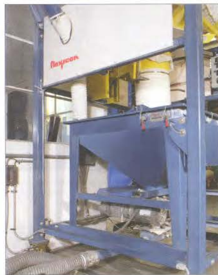
Below the hopper on the bulk bag discharger frame, a drop-through rotary valve meters PVC resin into two pneumatic conveying lines.
