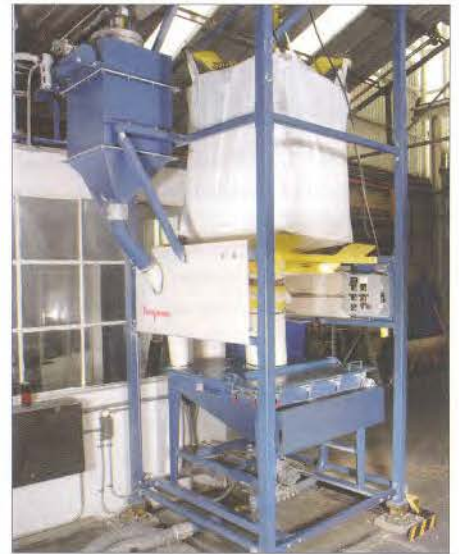
Oplex installed a BFC Series bulk bag unloader from Flexicon to improve the quality and productivity of its PVC compounding operation. Features include a cantilevered I-beam and hoist, Bag-Vac dust collector, Flow-Flexer bag activators beneath the bag for positive material flow, Tele-Tube telescoping tube and Spout-Lock clamp ring at the bag spout interface, hopper, and PLC-controlled rotary valve.
