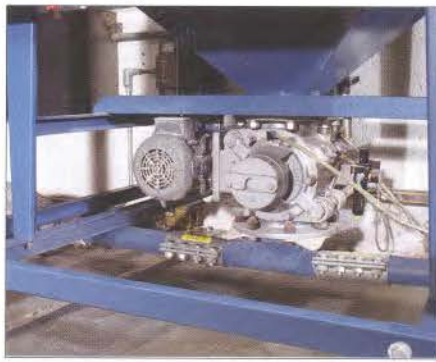
PVC from the bulk bag unloader is pneumatically transported to a 91.4cm diameter filter-receiver and hopper on the third floor of the Oplex plant. The flexible screw conveyor empties calcium carbonate into the smaller weigh hopper. Both ingredients are then gravity fed to the mixer on the floor below.
