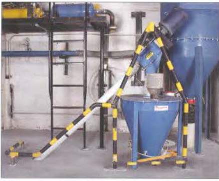
PVC from the bulk bag unloader is pneumatically transported to a 91.4cm diameter filter-receiver and hopper on the third floor of the Oplex plant. The flexible screw conveyor empties calcium carbonate into the smaller weigh hopper. Both ingredients are then gravity fed to the mixer on the floor below.
