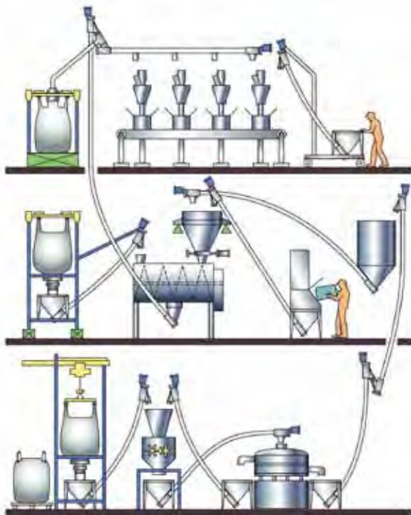
**Figure 1:** Properly engineered flexible screw conveyor systems can transport free-flowing and non-free-flowing bulk materials at any angle, through small holes in walls or ceilings. The screws and tubes of certain designs can be curved under, over or around obstructions, eliminating the need for exact conveyor routing.
