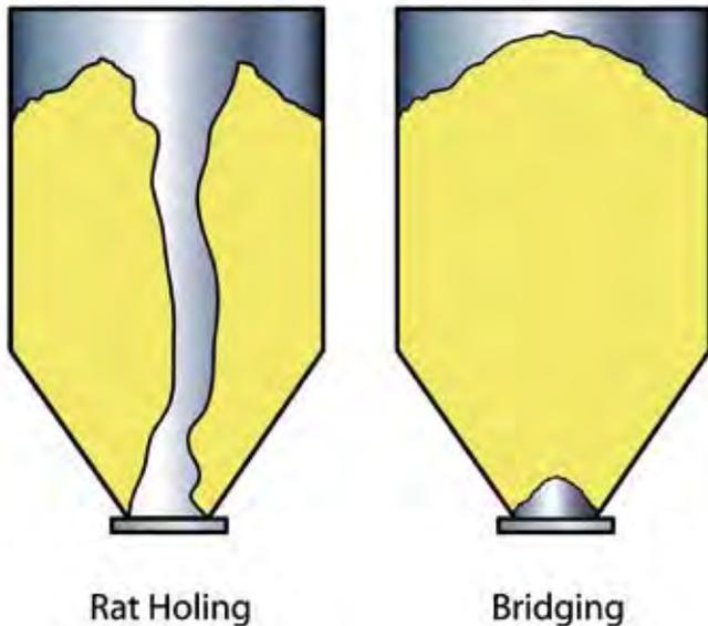
**Figure 3:** 'Rat-holing' (left) describes a ragged, tunnel-shaped void through stagnant material in the vessel. 'Bridging' (right), also known as doming or arching, describes a void area at the vessel outlet. Both rat-holing and bridging completely prevent the flow of material.
