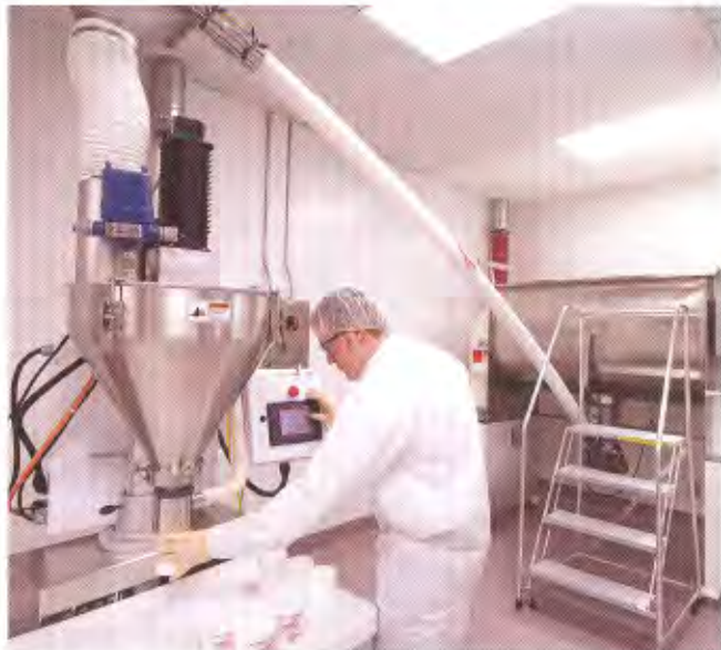
Due to space constraints, Macleod Pharmaceutical selected a Flexicon flexible screw conveyor to transport powder between a ribbon blender to a filling machine
