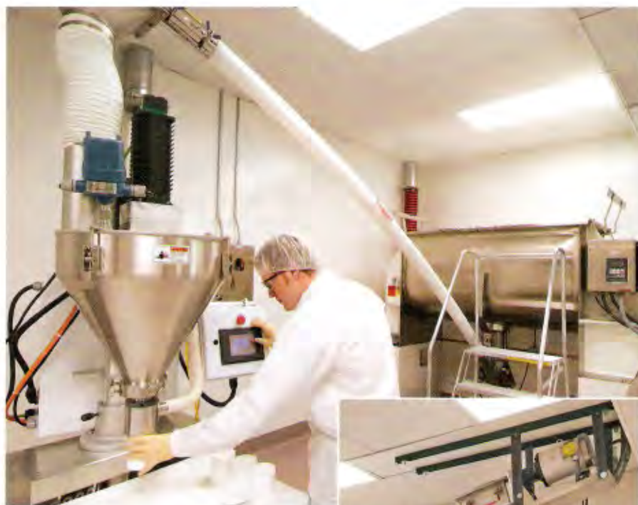
Flexible screw conveyors, like this Flexicon model, can use less space by conveying vertically in a tight footprint.
