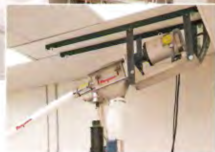
Flexible screw conveyors, like this Flexicon model, can use less space by conveying vertically in a tight footprint.
