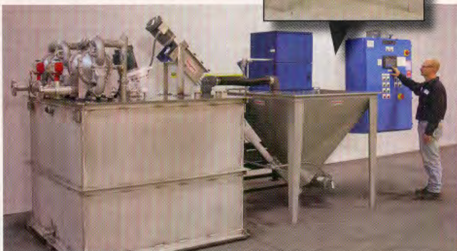
Oberlin Filter’s DMax filtration system features an automated dry chemical delivery system that provides more precise dosing than possible with manual methods. A hopper and flexible screw conveyor from Flexicon Corp. deliver dry treatment chemicals to the wastewater holding tank.
