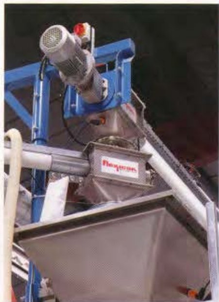
The first of three transfer points, a slide valve between the flexible screw conveyor and the hopper inlet opens and closes to regulate product flow.
