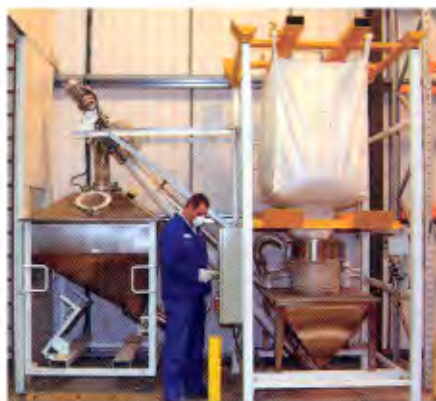
Fully enclosed system, comprised of bulk bag discharger, receiving hopper, flexible screw conveyor, and transfer bin, dramatically reduces operator exposure to airborne dust.
