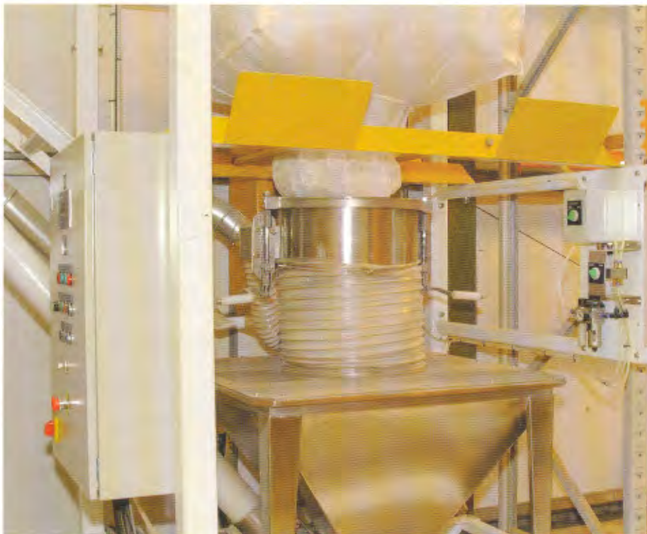
The Spout Lock™ clamp ring and Tele-Tube™ telescoping tube allow quick, dust-tight connections between bag spout and hopper and elongates bag as it empties to promote flow.
