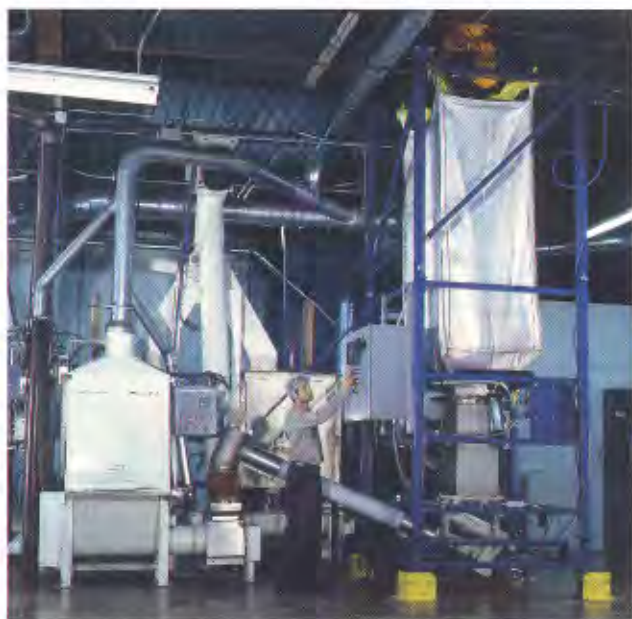
Automated bulk bag weigh batching system consists of 18'4" (550 cm) high discharger frame and 5-ft (150 cm) long flexible screw conveyor. Under loss-of-weight control, the system discharges precise amounts of powder into an auger conveyor that feeds three ribbon blenders.
