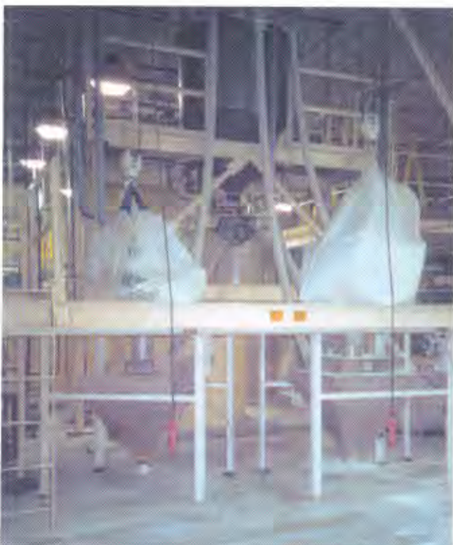
Flexicon flexible screw conveyors move three forms of feldspar from individual hoppers to a single weigh hopper at the Lenox China's manufacturing plant
