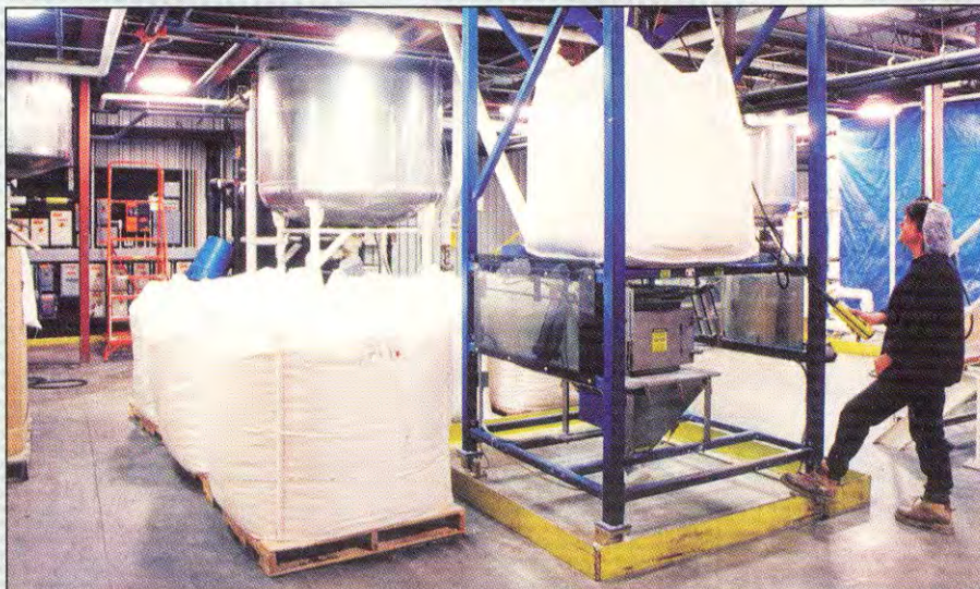
Bradford Soap redesigned its material handling system from manual bag dumping to automated bulk bag unloading, and added a flexible conveying system to increase production.
