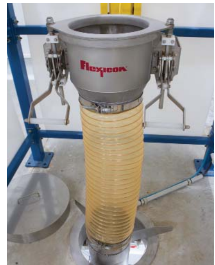
The Spout-Lock™ clamp ring creates a sealed connection between the clean side of the bag spout and the clean side of the Tele-Tube™ telescoping tube, which raises the clamp ring for connection to the bag spout and then lowers, applying continual downward tension to promote flow into packaging machine on the floor below.
