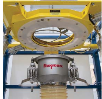
Operator pulls the bag spout through the Power-Cincher™ flow control valve in which four elliptically contoured bars cinch the bag spout concentrically, enabling partially emptied bulk bags to be retied and removed.
