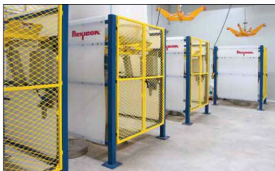
Four of Prosur's seven Bulk-Out® model BFH-C-X half-frame bulk bag dischargers: an electric hoist positioned over each discharger lifts the filled bags on to the half frame.
