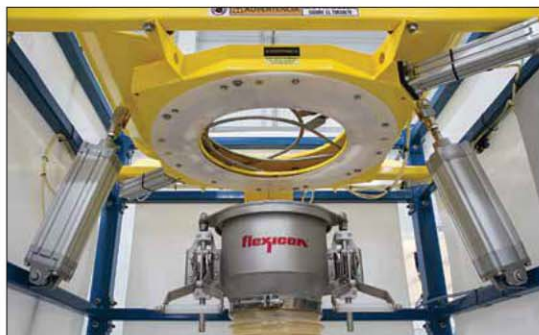
The Power-Cincher flow control valve closes the bag discharge spout concentrically, allowing partially emptied FIBCs to be retied and removed (see front cover picture).
