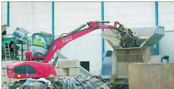
A Jupiter 2200 shredder from Lindner-Recyclingtech shown being loaded with unclean agricultural film at the Zutphen, Netherlands, waste processing plant of Daly Plastics; the shredder is said to offer the perfect cut as well as safeguarding against foreign objects, helping to produce plastic regranulate which is comparable to virgin material (see article on p12).
