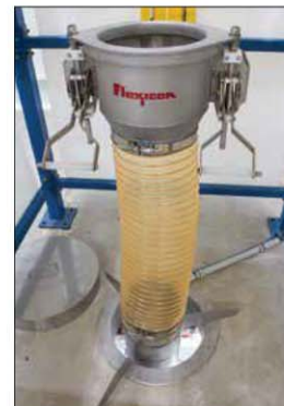
The Spout-Lock clamp ring creates a sealed connection between the clean side of the bag spout and the clean side of the Tele-Tube telescoping tube.
