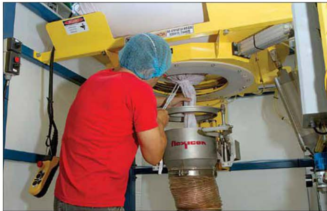
One of seven Flexicon bulk bag dischargers recently installed at the Spanish food processing plant of Productos Sur (see p13); an FIBC discharge spout is shown clamped shut by the Power-Cincher flow control valve, allowing partially emptied bags to be retied and removed.
