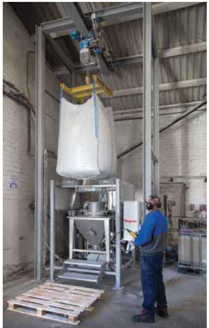
The cantilevered hoist and trolley position the bag for discharge into the 226 l hopper and through a rotary valve into the pneumatic line.
