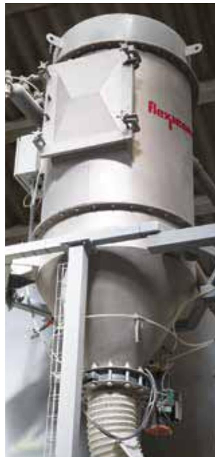
From the pneumatic line, the filter-receiver separates the mineral powder from the air stream before discharging the powder into the extruder. System operation is under PLC control.
