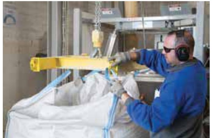
Operator delivers bulk bag, and attaches bag loop straps to the lifting frame.
