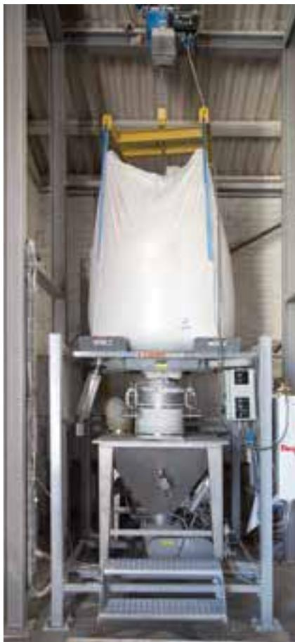
The powder flows dust-free into the hopper and into the 38 m long pneumatic transfer line.
