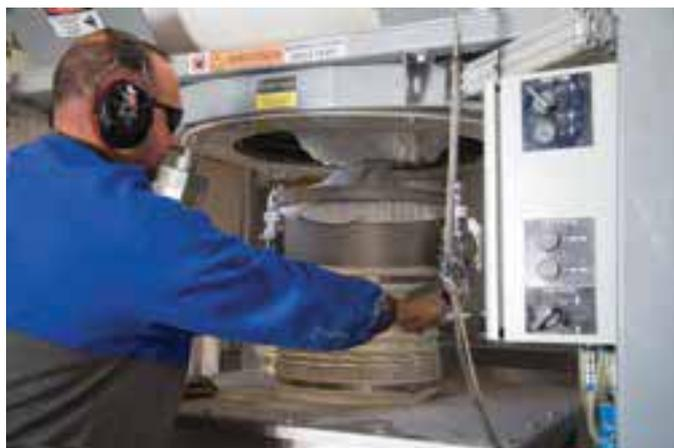
The operator pulls the bag spout through the Power Cincher flow control valve which prevents product leakage and facilitates tying off a partially empty bag.
