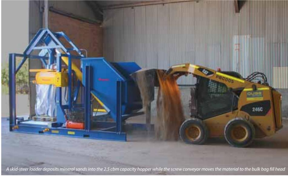
A skid-steer loader deposits mineral sands into the 2.5 cbm capacity hopper while the screw conveyor moves the material to the bulk bag fill head
