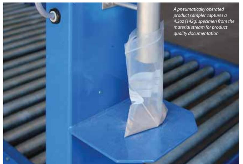
A pneumatically operated product sampler captures a 4.3oz (142g) specimen from the material stream for product quality documentation
