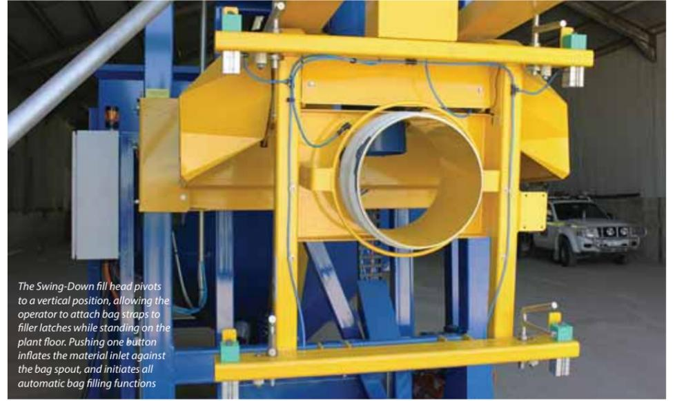
The Swing-Down fill head pivots to a vertical position, allowing the operator to attach bag straps to filler latches while standing on the plant floor. Pushing one button inflates the material inlet against the bag spout, and initiates all automatic bag filling functions
