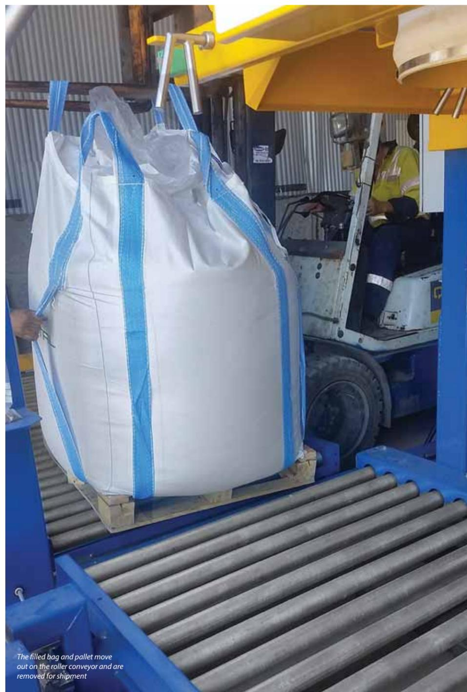
*The filled bag and pallet move out on the roller conveyor and are removed for shipment*
